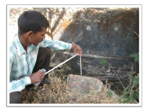
A Jaldoot taking ground water measurement with measuring tape
